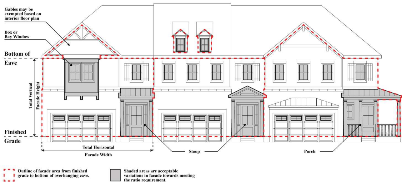
Illustration 11. 5: Front façade area measurements
