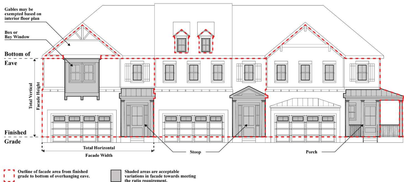
Illustration 11. 5: Front façade area measurements
